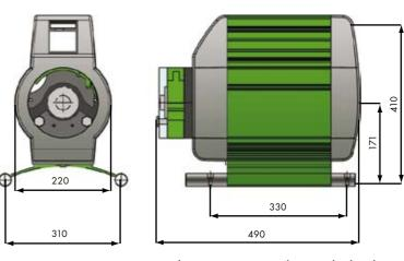
The S30 Pump Head is supplied with a saddle for a 3.2mm wall thickness tube as standard
