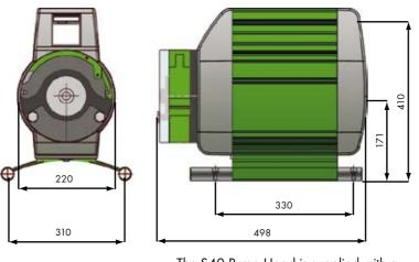
The S40 Pump Head is supplied with a saddle for a 4.8mm wall thickness tube as standard
