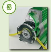
Open up the lever and fit the claw over the other set of dowels
